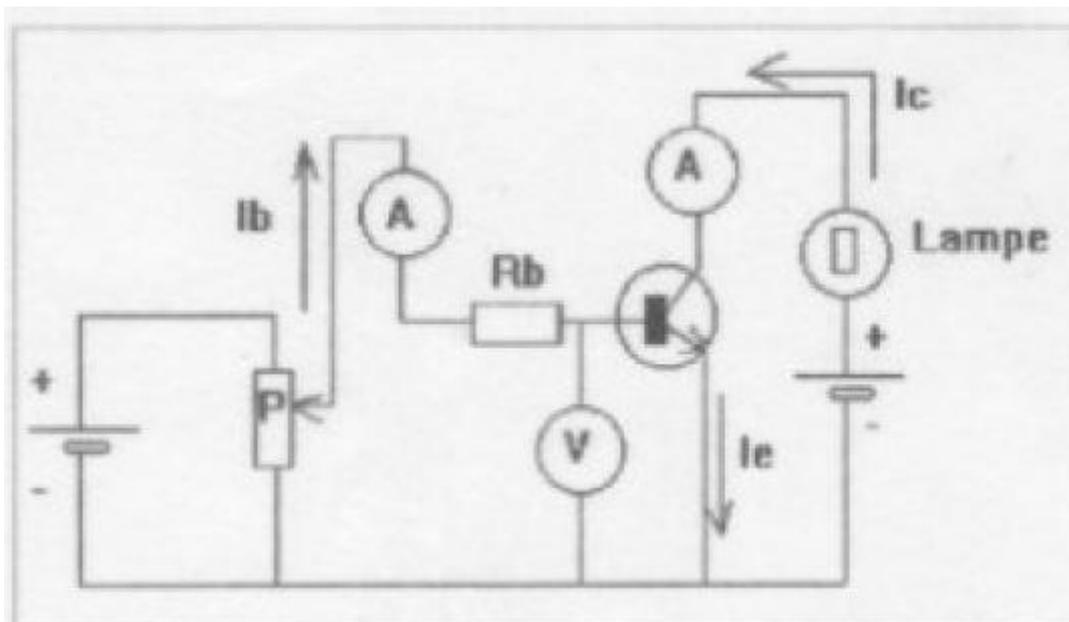
$I_c = 50 \text{ mA}$     $I_b = 1 \text{ mA}$
